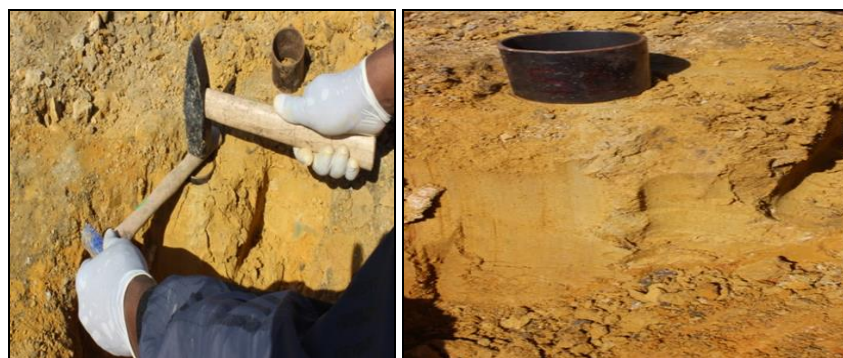
Fig 1: Taking soil samples from the different depths using soil cores
