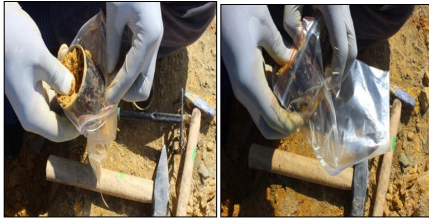
Fig 3: Emptying the soil sample inside the soil core to the plastic bag
